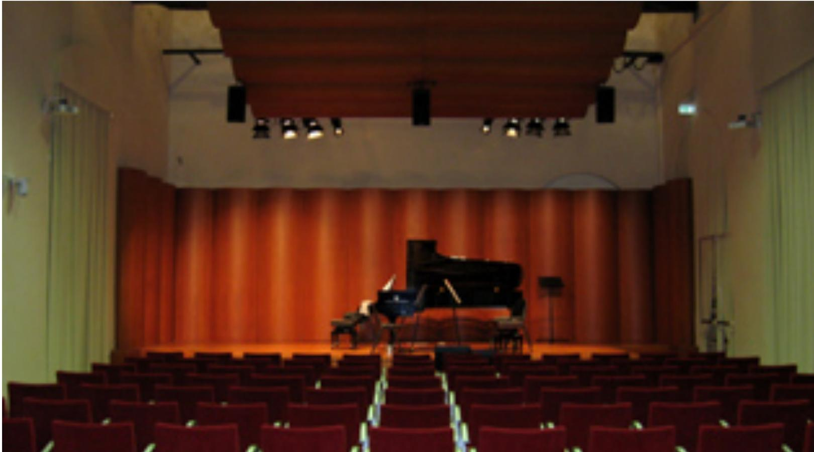
The Concert Hall consists of a listening space for 156 people whose sound diffusion is made up of three pairs of loudspeakers placed on the sides of the stalls, three loudspeakers of greater power placed above the stage and a mobile subwoofer.
